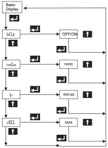
Structure of command menu for Resistance & Continuity measurement
